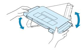
**18** Place the toner cartridges on a flat surface as shown and remove the paper covering on the toner cartridge by removing the tape.
